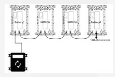
The matching address must select battery 1 as the host, and long press and hold its reset button for 15s. Do not select and press the reset button of other slave batteries. This step is particularly important as improper operation may result in battery networking failure.
